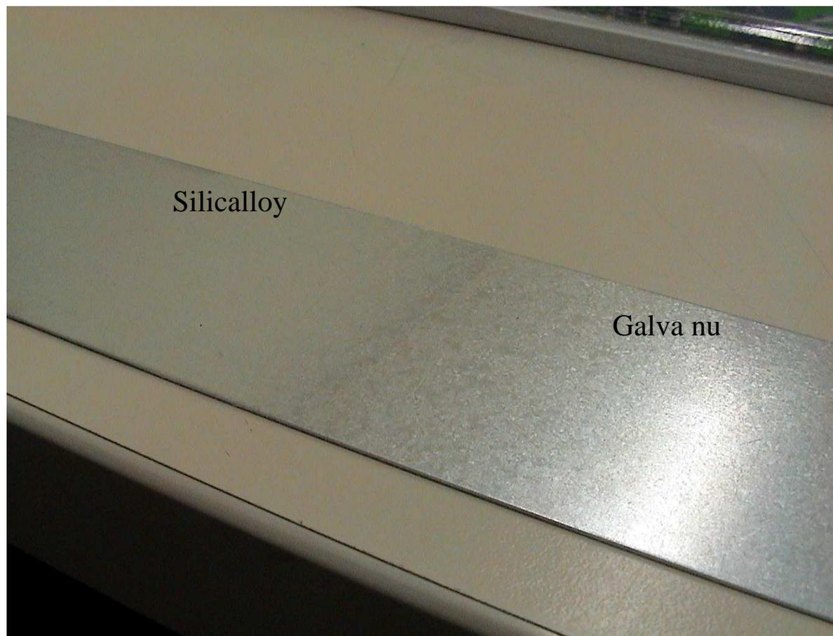
**Tests de passivation**
